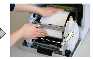
7. Set the ribbon into the printer. Unite and insert the position of the shape of a concave and convex form of an attachment and a holder.
