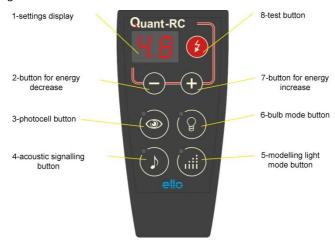
There are almost no differences between maintenance of lamp by means of control panel and of main front panel of the lamp. There are the same symbols that make the maintenance easy. Each press of button causes mode and signalling change. Energy control element consists of two buttons "-" and "+", instead of revolving potentiometer, for utilitarian conditions. Each press (7) or (2) button makes energy increased or reduced by 1/10 f-stop. Control panel is equipped with cable 10 m long.
